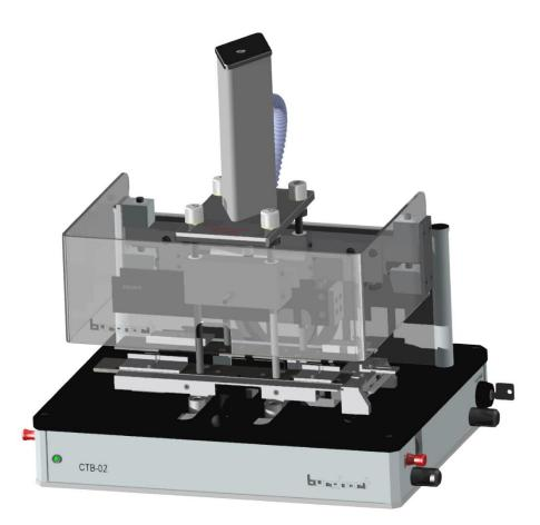
The CTB-02 is a measuring device to measure the restoring forces of cigarette pack creases after folding.
