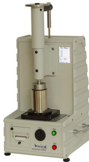
DD60A equipped with the Set for filling power measurement
