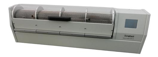
The Ends Tester E44 A is used to determine the loss of tobacco from the cigarette ends with or without filter. For this purpose, the E44 A simulates the rolling and rubbing movements of the cigarettes during production process. The E44 A works in accordance with ISO 3550-1.
