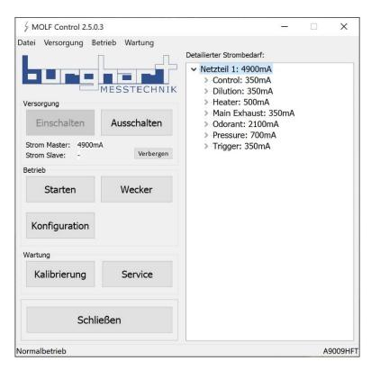
The olfactometer is operated via its own software (MolfControl). Dialogue-guided standard procedures support the user in the proper use of the programme. This improves usability and ensures intuitive operation.
