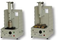
DD60A measuring filling power and/or hardness
