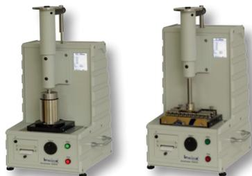
DD60A measuring filling power and/or hardness
